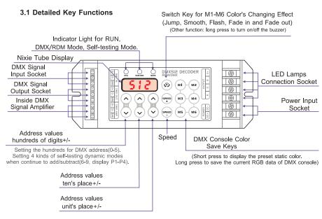
In the DMX Decoder Mode, the "RDM/DMX" indicator light is on, the "RUN" indicator light flash quickly if RDM/DMX signal input. In the self-testing mode or editing dynamic effect mode, the "MODE" indicator light is on.
